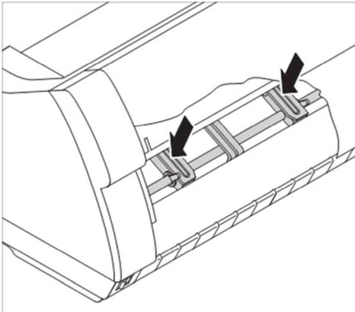
Check that any paper has been removed from the tractors.
