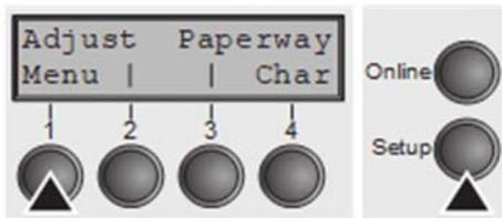
Press the **Setup** key. The printer switches to Setup mode. (can be selected both in the Online and Offline mode). To access the printer menu, press the key directly underneath the word **Menu** (1).
