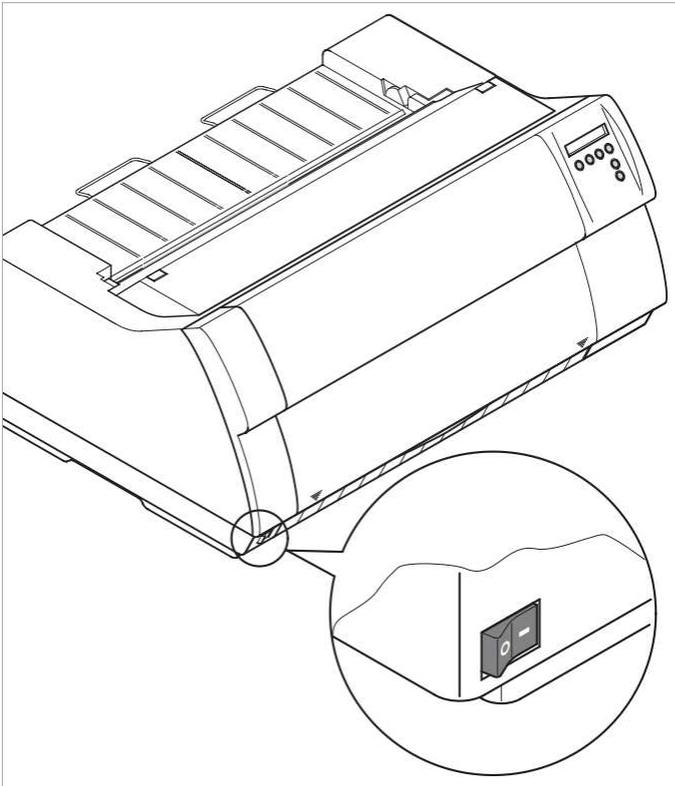
The power switch for switching on the printer is located at the bottom left at the front of the printer when viewed from the front.
