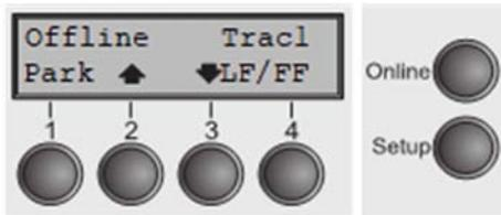
Make sure that the printer is in offline mode; press the **Online** key, if necessary.
