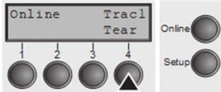
Make sure that the printer is in online mode. If necessary, press the **Online** key.
