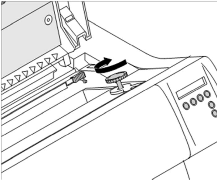
Insert the coloured tension knob into one of the two locations.
