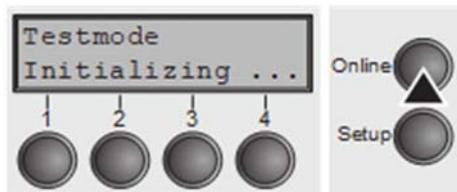
Enter advanced menu mode by pressing the key **Online** while switching on the printer.
