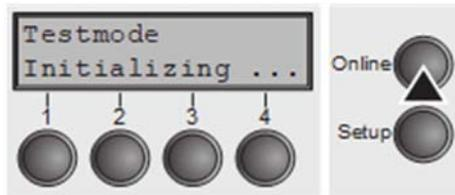
The display shows **Test mode** for approx. 1 second and then automatically changes to display **ASCII 80 ASCII 136**.
