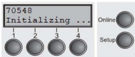
If the memory test is successful finished, the firmware number appears in the display.
