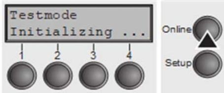
Before performing a self-test, your printer must be switched off. Ensure that paper is inserted. Keep the key **Online** pressed while switching on the printer, until **Testmode** appears on the display.
