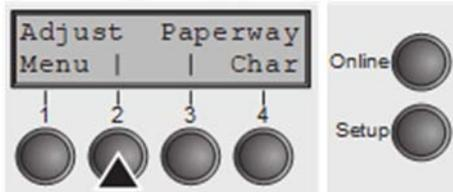
Press the **Setup** key. The printer changes to setup mode.
