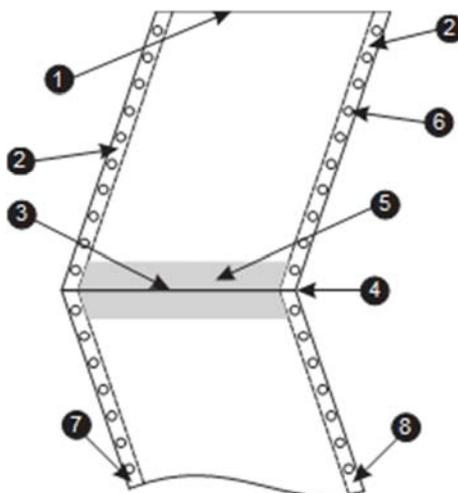
If the parameter is set to **On**, the printhead gap increases during form feed and line feed four lines before and after the perforation on the form (= protected zone). The printhead gap is always increased during form feeding past the perforation even when feeding takes place outside the protected zone.
