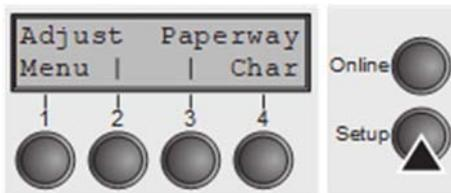
Press the **Setup** key. The printer returns to the initial status.
