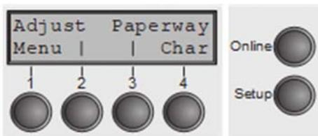
It is also possible to change to Setup mode when you are in Rolling test mode if you want to change the configuration for the test printout.
