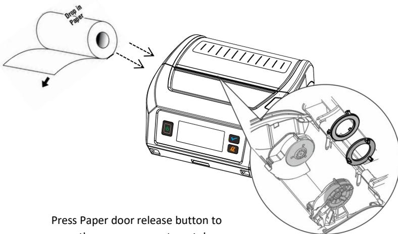
Press Paper door release button to open the paper compartment door. Pull small leader of paper out and close paper door. "Clicks" when properly closed.
