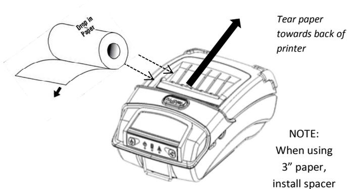
Press Paper door release button to open the paper compartment door. Pull small leader of paper out and close paper door. "Clicks" when properly closed.
